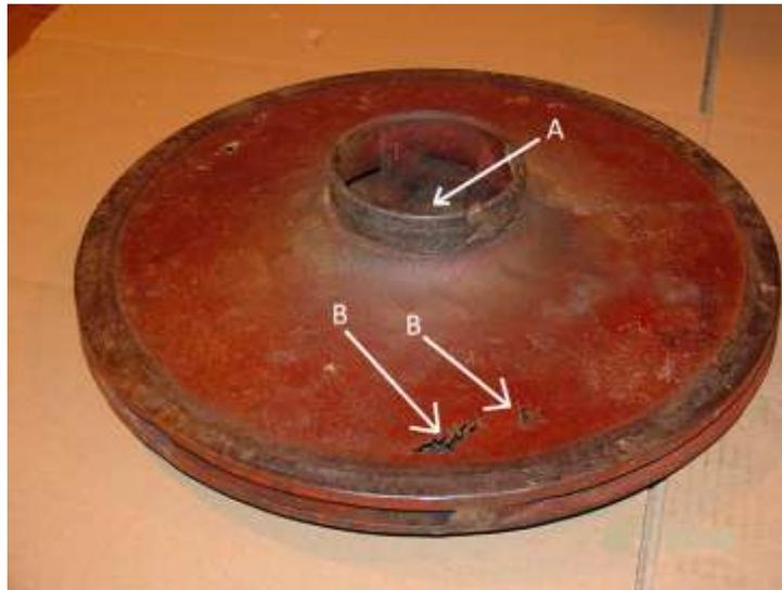
The dark spots in the photo above (indicated by the 'B' arrows) are holes in the impeller. Bubbles form in the low pressure area at the center of the impeller (above, point A). These bubbles flow with the water out to where the pressure is higher. Here they implode and cause damage (above, points B).
